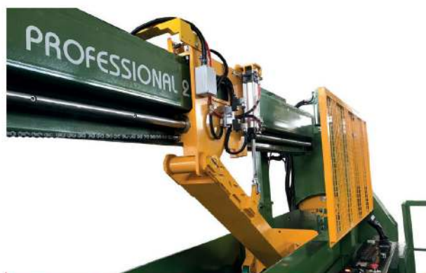
Lifting pusher with mechanical/pneumatic system
