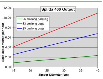
chart is based on continuous ne machine when processing a ber diameters at the lengths quoted in solid cubic metres
