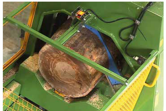
Photocell for automatic log length measurement
