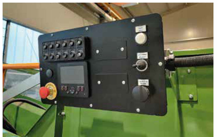
K650 - Control panel
