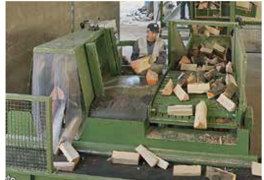
11 Ton splitting station, 2+4 folds grid
