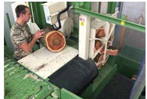
20 Ton splitting station, 2+4+6 folds grid
