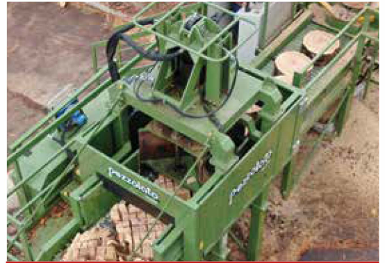
Automatic vertical splitter
