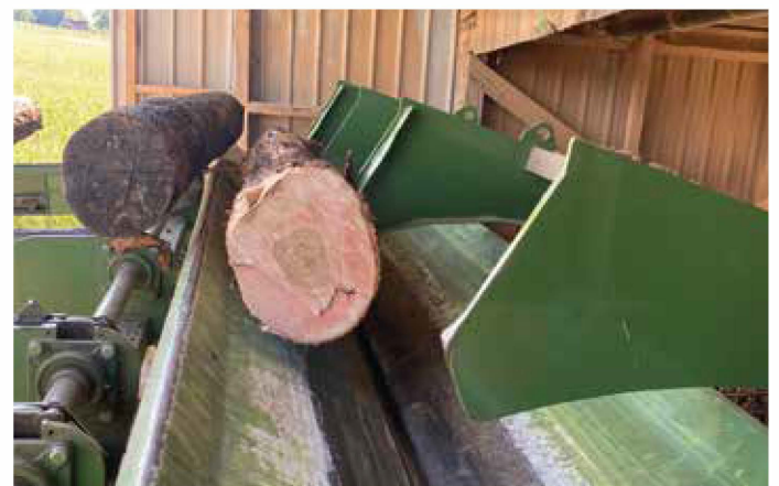
Log loader and damper arm
