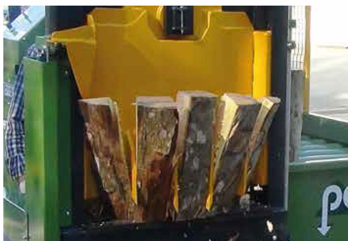
Wedge with 4 orbital blades producing 5 logs per cycle
