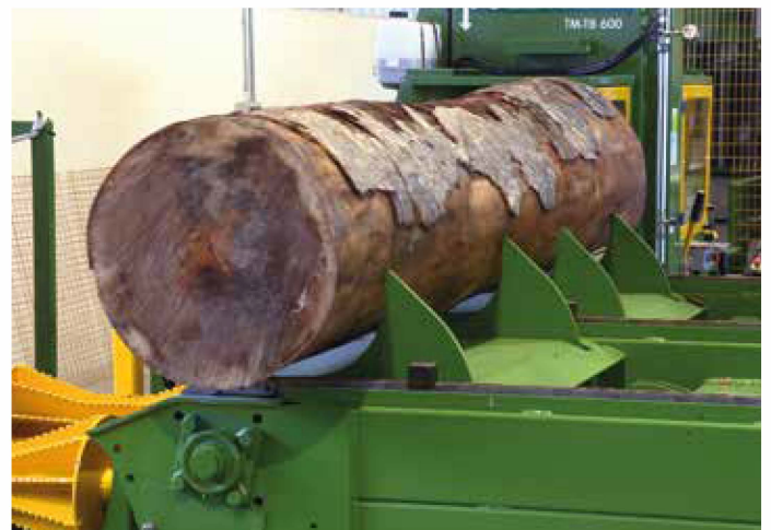
3-chain loading deck, 4 meters in length
