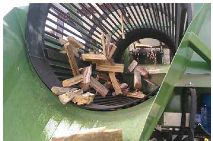
Drum screener for bark and residual sawdust
