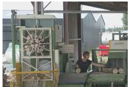
32 Ton splitting station, 2+4+6+16 folds grid
