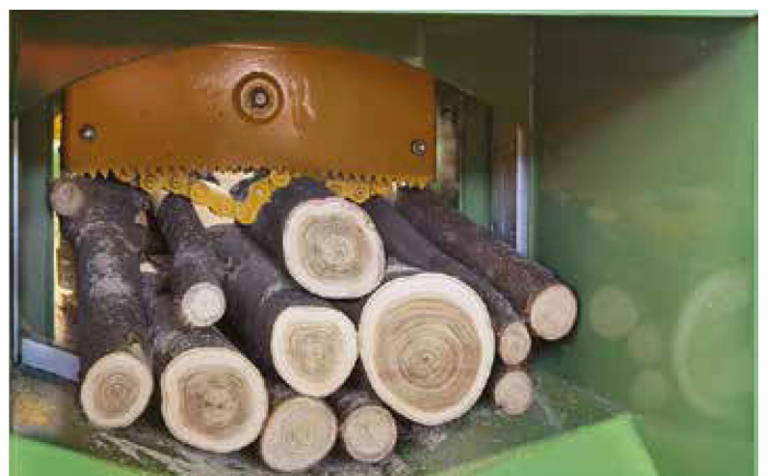
Chain locking system. Efficient on all species of bundles
