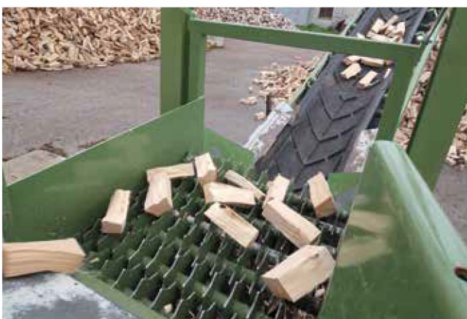
Cleaning rollers for bark and residual sawdust
