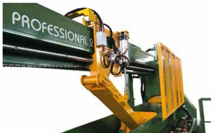
Lifting pusher with mechanical/pneumatic system
