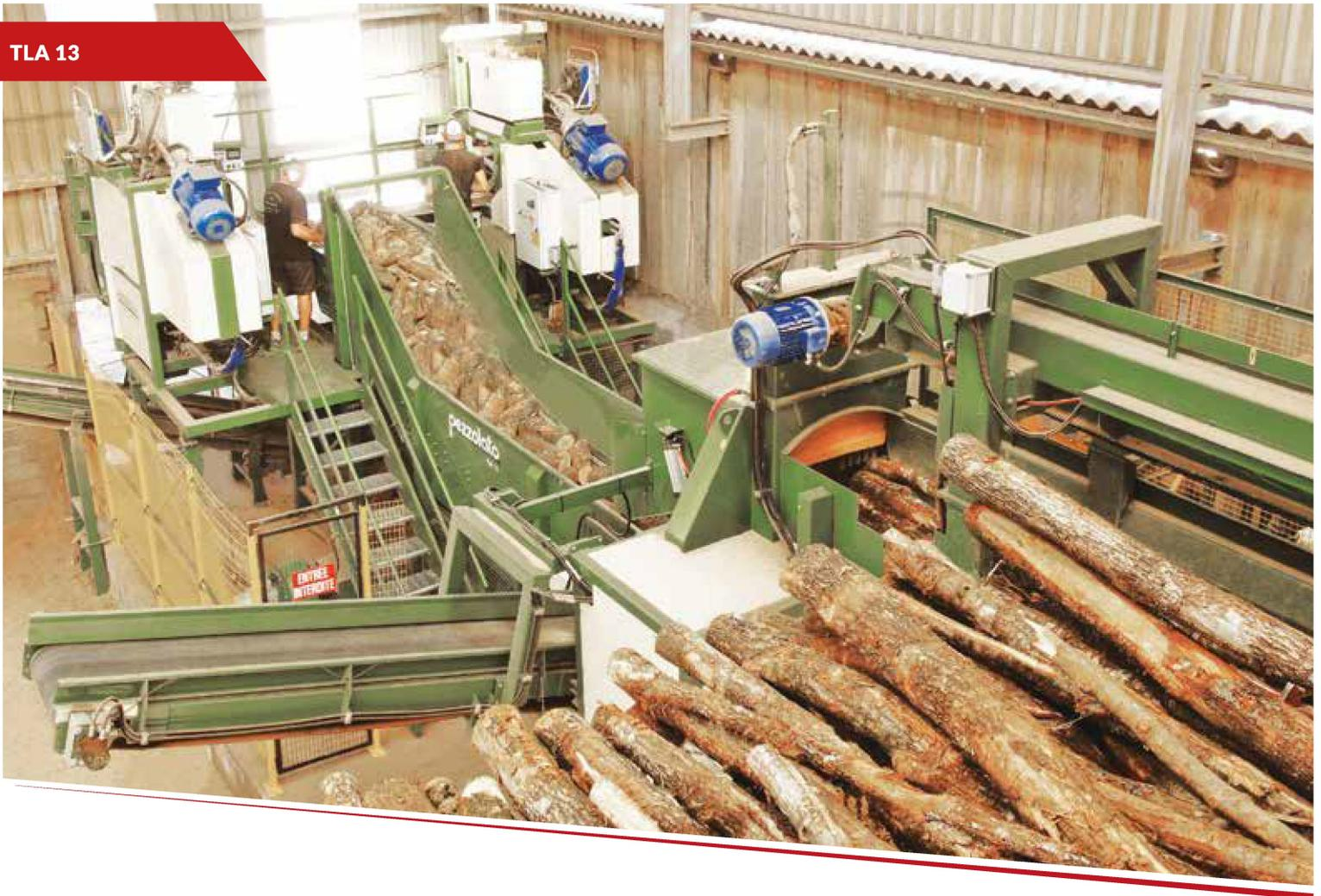
After cutting, the logs fall in a cumulating S-shaped conveyor (with closed meshes), which transfers them in front of the wood splitter.
