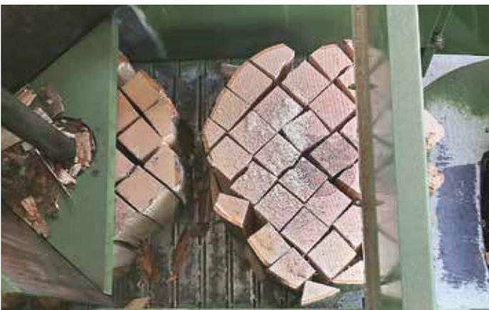
Wedge for automatic vertical splitting system
