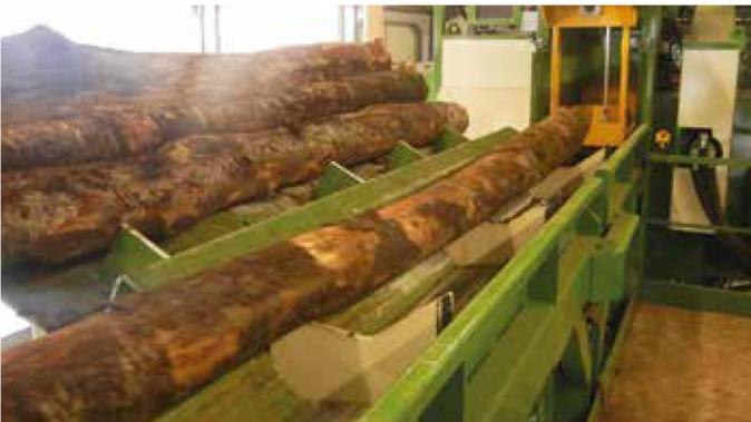
Loading system with step-feeder
