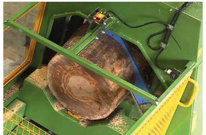
Photocell for automatic log length measurement
