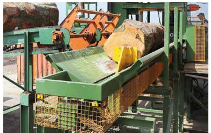
Feeding tube with rear pushing unit
