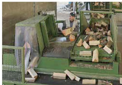
11 Ton splitting station, 2+4 folds grid
