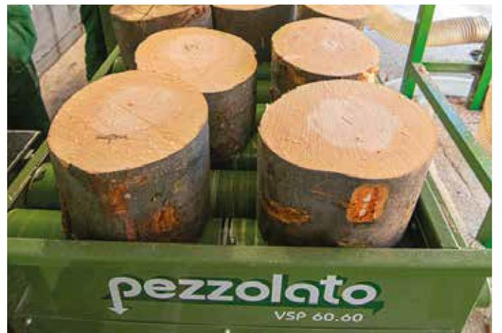
Motorized rollers table for transferring cut logs
