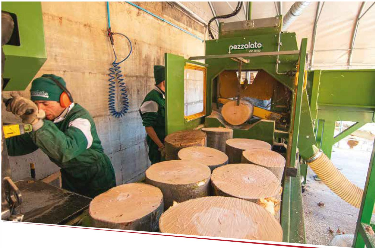
The manually operated hydraulic double log splitter with a thrust force of 20 tonnes consists of a curved wedge with four orbital knives that allow five logs to be split per work cycle.
