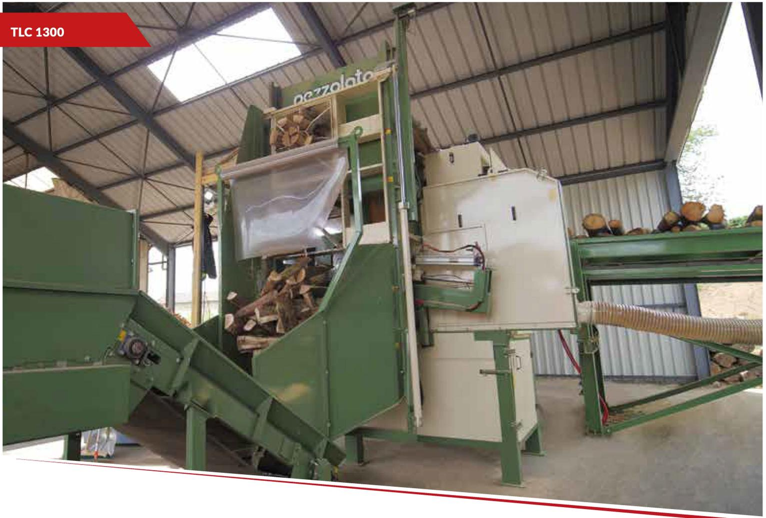
By choosing the automatic cut/split cycle, the splitting grid moves automatically according to the diameter of the log to be processed.
