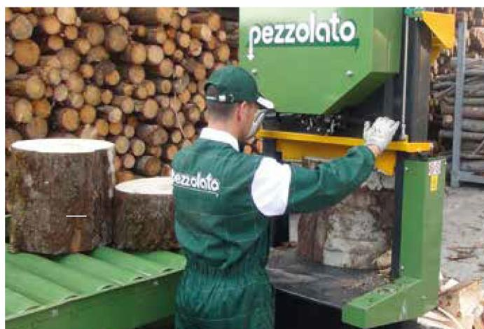
Double manual hydraulic control for wood splitter Wedge
