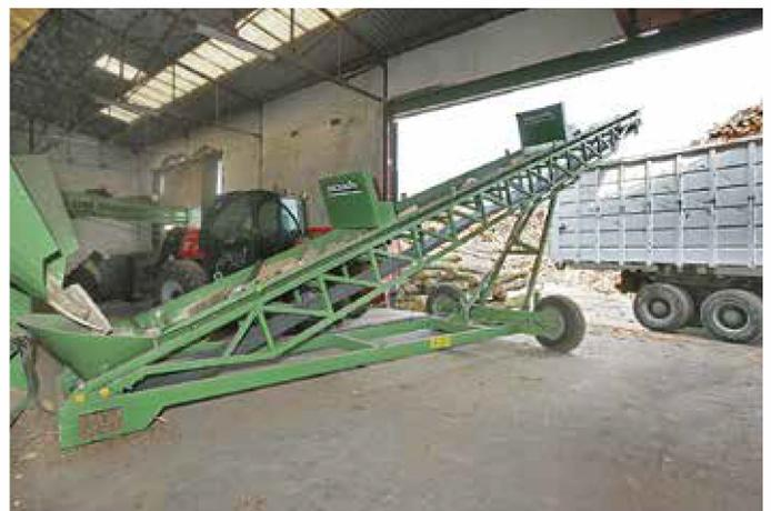
hydraulic orienting for conveyor with wheels
