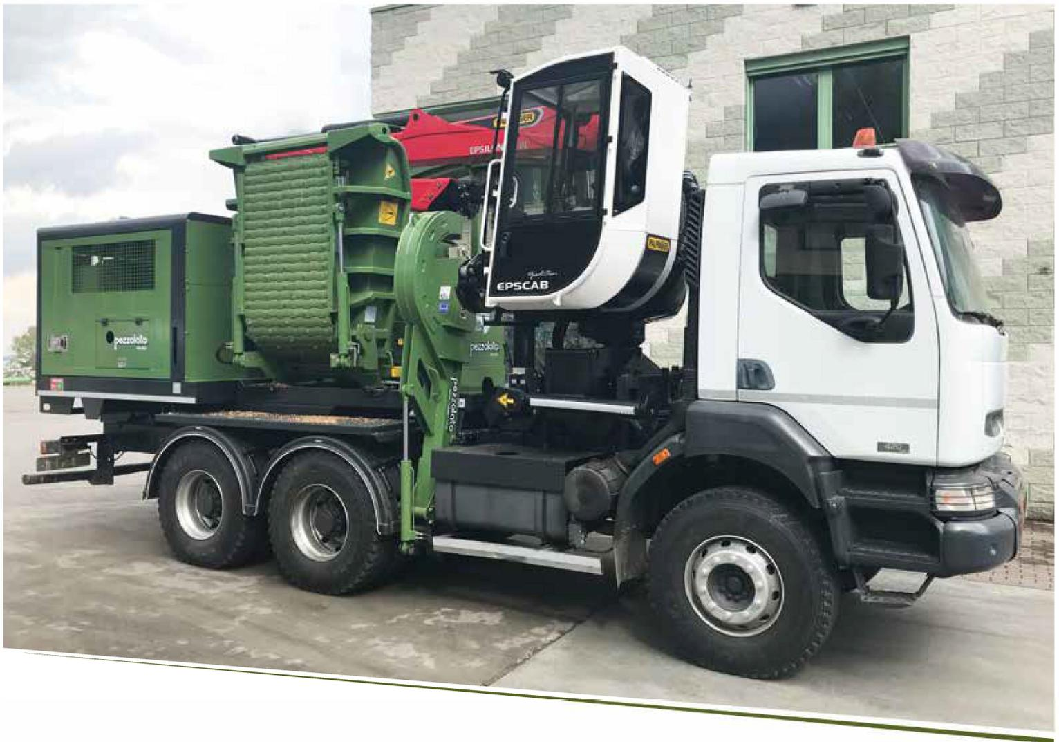
The large fan (1250 mm) mounted directly on the drum shaft is able to work at a low speed (less than 600 revs) to help reduce dust and increase wood chip quality.
