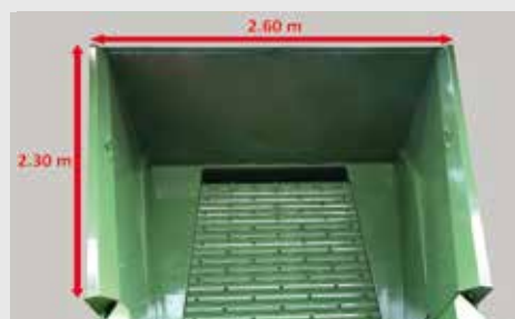
Dimensions accumulation hopper PTH 1200/1000
