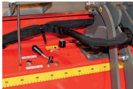
The AC 10 automatic chain tensioner maintains optimal saw chain tension at all times. The chain can be conveniently replaced after releasing chain tension with the lever pictured – no tools required!
