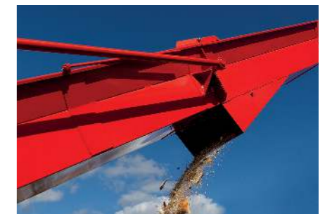
Patented cleaning outfeed conveyor as standard. The groove at the end of the outfeed conveyor separates debris from the firewood.
